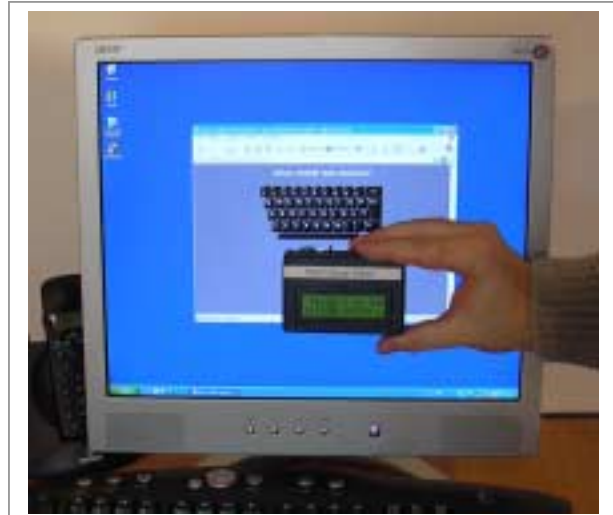
The Silicon Wallet can get text from a web browser by means of a phototransistor
