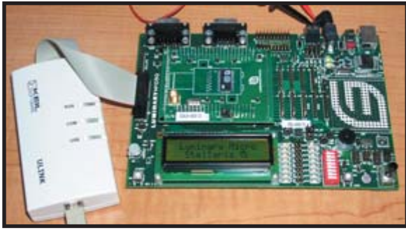
Photo 2 —The Stellaris development kit comes with a lot of stuff (a board, JTAG debugger, and software tools) and a price to match. If you're on a budget, one alternative is to just use the $190 part-specific daughter-board. Or, for that matter, rolling your own prototype is an option thanks to the chip's relatively spacious 0.05" pin pitch.
