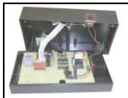
Photo 1 —The prototype was wire-wrapped and installed in a 5" x 7" plastic box. The high-voltage components are along the right side next to the battery compartment.
