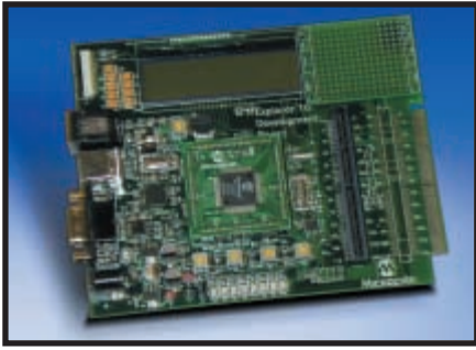
Photo 1 —Success in the MCU mass market calls for more than a good chip. Microchip carries that lesson learned long ago forward with their $130 Explorer 16 evaluation board, which supports all the members of the dsPIC and new PIC24 families.
