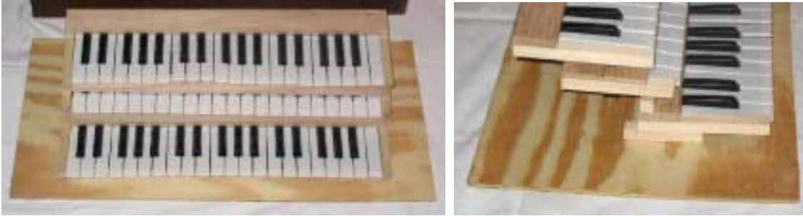
Three Tier Keyboard Prototype Front and Side View with 95 Keys
