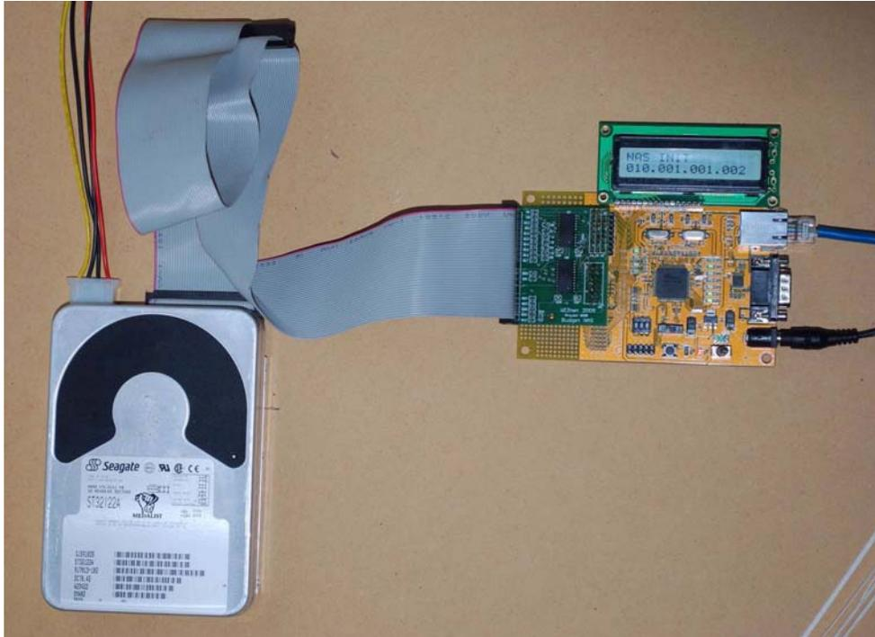
Figure 3. Unit Operating with IDE HDD
