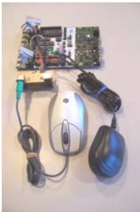
The AVR STK500 Starter Kit with a block of four PS/2 connectors scavenged from an old KVM switch. The power supply is used to power the mice via the PS/2 connectors.
