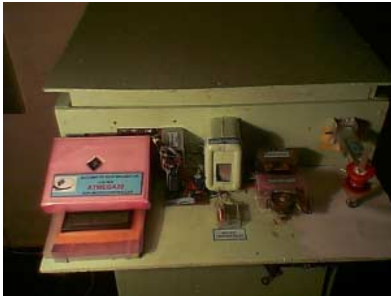
(Figure shows the full system view. Main Controller board is inside the rose box. ATMEGA32 can be seen through the slit. Figure shows other parts of the system)
