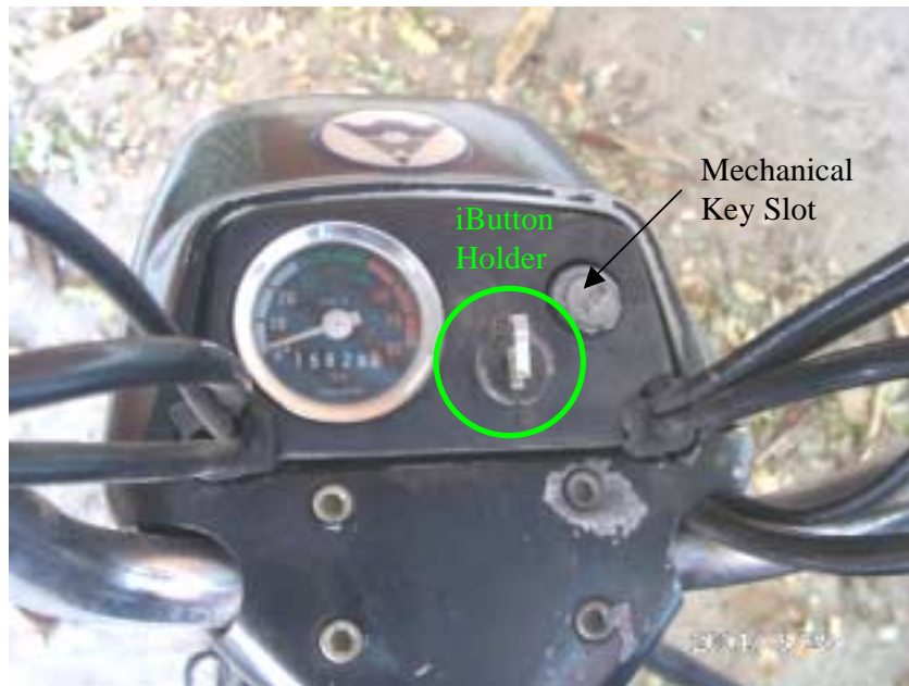
Figure 3: VSS mounted in two-wheeler
